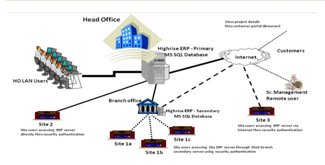
Remote/ Site/ Branch Users can access directly or via internet via VPN, MS remote
