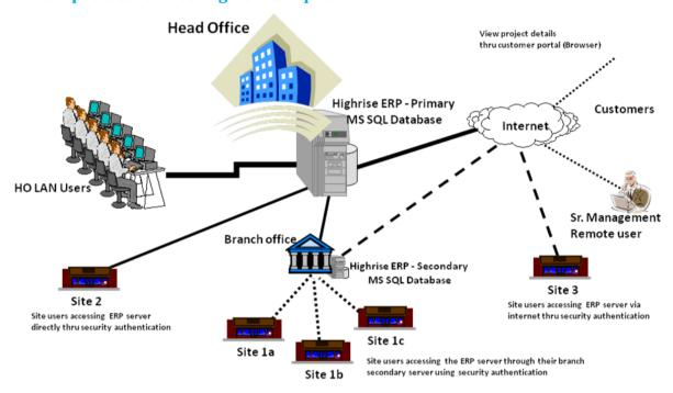
Remote/ Site/ Branch Users can access directly or via internet via VPN, MS remote
