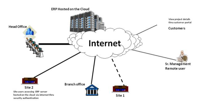
Remote/ Site/ Branch Users can access ERP Server hosted on the cloud at Hosting Service Provider
