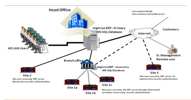
Remote/ Site/ Branch Users can access directly or via internet via VPN, MS remote Desktop
