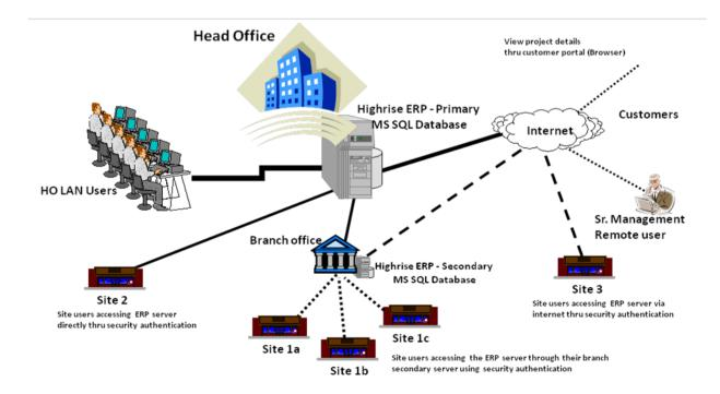
Remote/ Site/ Branch Users can access directly or via internet via VPN, MS remote Desktop Terminal Client or Browser
