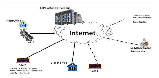
Remote/ Site/ Branch Users can access ERP Server hosted on the cloud at Hosting Service Provider
