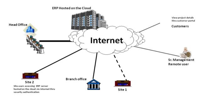
Remote/ Site/ Branch Users can access ERP Server hosted on the cloud at Hosting Service Provider
