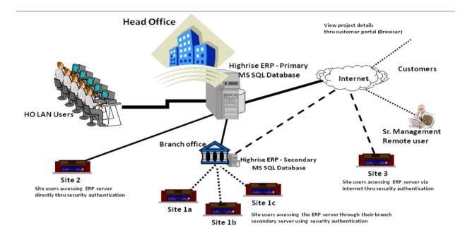
Remote/ Site/ Branch Users can access directly or via internet via VPN, MS remote Desktop Terminal Client or Browser
